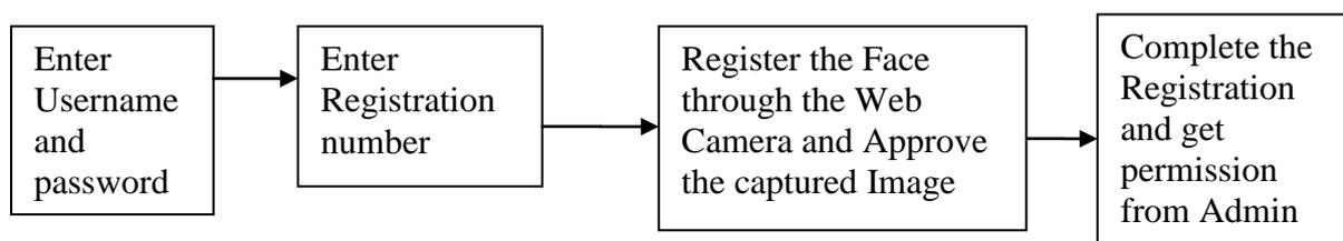
Figure 1: Steps involved in the Registration Procedure
